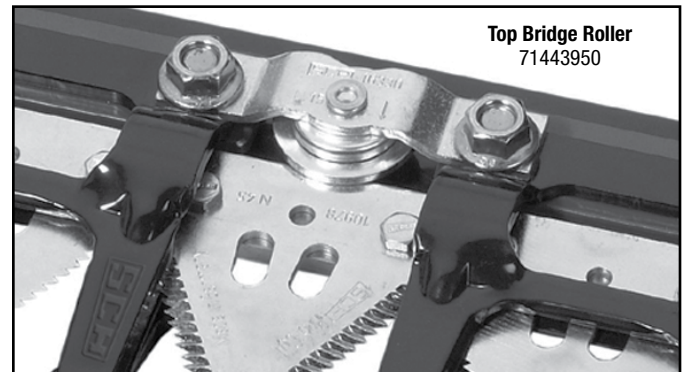
Top Bridge Roller holds knife straight to prevent section from tipping downward
