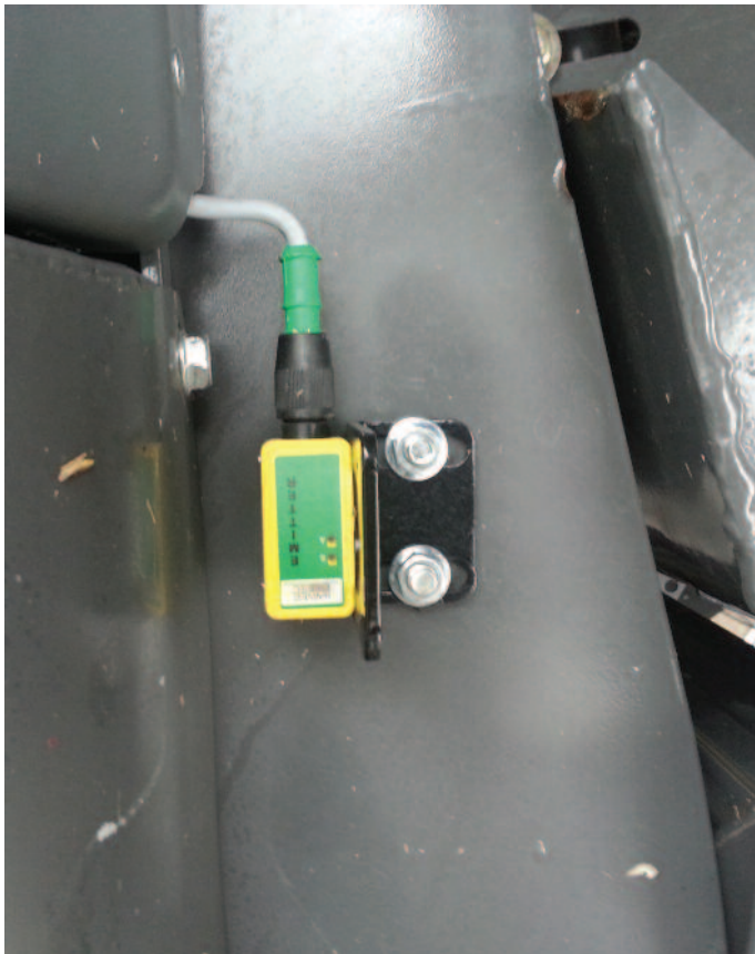
Crop eyes can be added as an option to automatically pause the applicator when no crop is passing over the pickup
