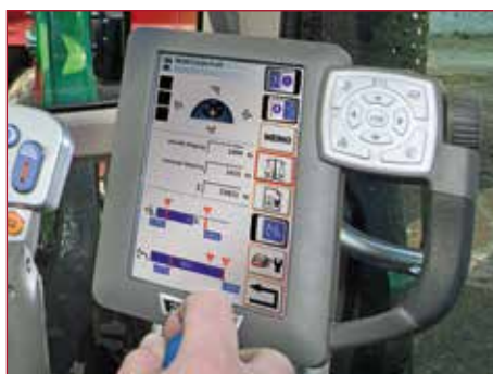
The settings for the CargoProfi are adjusted easily and intuitively with the Varioterminal.
