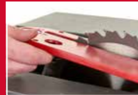
Anti-kick-back pawls stops material kicking back at the operator
