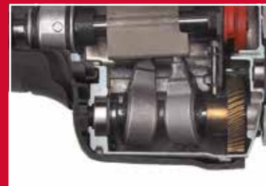
Counter balance mechanism ensures low vibrations - 12.5 m/s²
