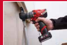
Right angle head for confined spaces
