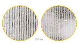
Competitor's moulding process allows material displacement, greatly reducing resilience and hampering performance.
