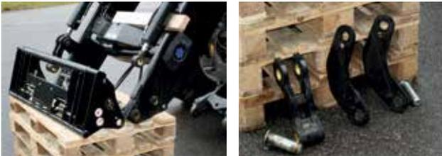
**IMPORTANT!** Although hydraulics are depressurized, the cylinders may extend slightly causing pinching. Also, you may need to adjust the length of the cylinder to get the holes aligned. This is easily accomplished by using a crowbar.
