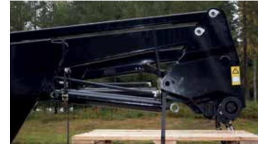
Place a piece of wood (or rubber pin locking) between the parallel link and the arm before knocking out the middle pin. Pivot the bearing box backwards and reinsert the pin in the hole in the bearing box so that the pin acts as a wedge. Replace the bushings and refit the middle pin.
