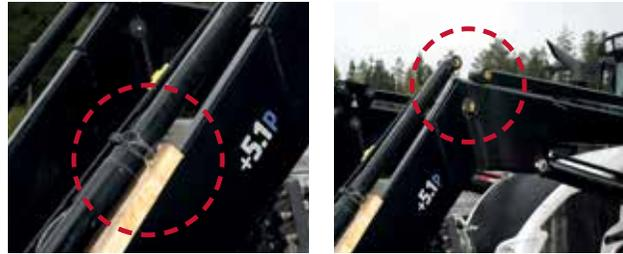
Be careful not to drop the triangle links on the ground. Replace the bushings. Assemble and move on to Step 3.
