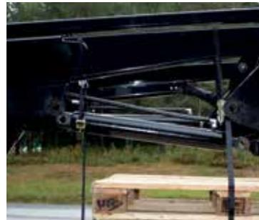
Reassemble the front pin, but allow the rear part to continue to hang in the strap. Remove the top pin on the bearing box (parallel link) so that the bearing box is hanging on the middle pin. Angle the bearing box so that it is possible to replace the bushings in the top hole, and then immediately reinstall the pin.
