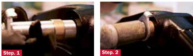
▲ **Step 1.** Thread the bushing on to the pin.
