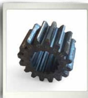
Teeth surface deteriorated due to poor quality heat treatments
