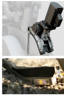
Figure 6. Variable Depth Moisture Control mode in the Precision Planting 20/20 Gen3 monitor (left), Precision Planting SmartDepth gearbox for real-time adaption of planting depth according to soil moisture (top right), and Precision Planting SmartFirmer for measurement of soil moisture in the furrow (bottom right).
