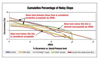
The table below shows the products tested listed in the order of the number of noise events. By studying this table and the adjacent graph, it can be determined that, during these tests, LOCTITE® Disc Brake Quiet Stick was the most effective at reducing brake noise events.
